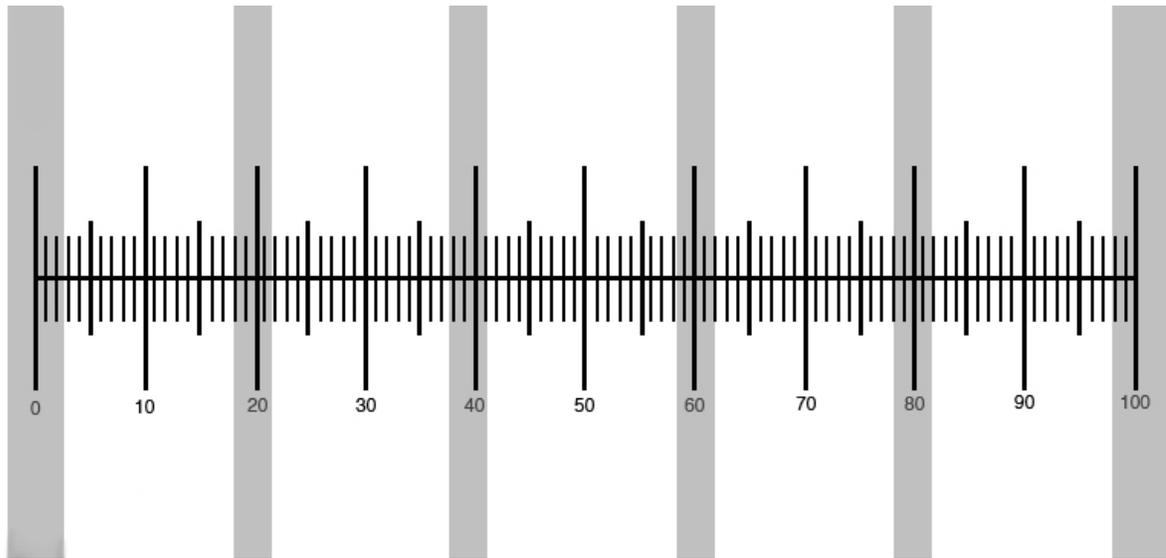
**Fig. 2.3 - Ocular micrometer superimposed on stage micrometer: In this case the lines of the stage micrometer appear much broader than those of the ocular micrometer due to the increased magnification. The exact distance between ocular divisions is 0.001mm or 1 micrometer ( $1\mu\text{m} = 1 \text{ micron or } 1\mu$ ).**
