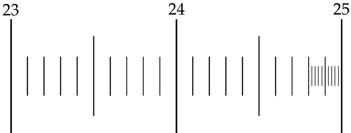
**Fig. 2.2 - Stage Micrometer: On the metric scale, lines 1 - 25 are spaced exactly 1mm (1000 $\mu$ m) apart, the lines between 24 and 25 are spaced 0.1mm (100 $\mu$ m) apart, and the smallest lines (far right) are spaced 0.02mm apart. Note - 0.02 mm = 20 micrometers (20 $\mu$ m) = 20 microns = 20 $\mu$ .**
